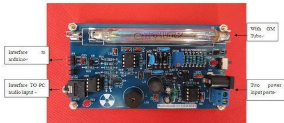
Figure-8: Geiger- Muller Counter connection points [3]
